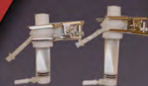
Dry Heat Bubble Free Cells (DHBFC) designed to test creams, lotions, ointments and patches
