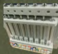
Syringe pump sampling system accuracy of \pm 1\%
